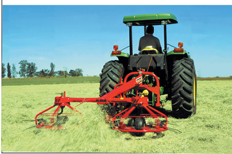
Rake turns when it works and locks when it is lifted
